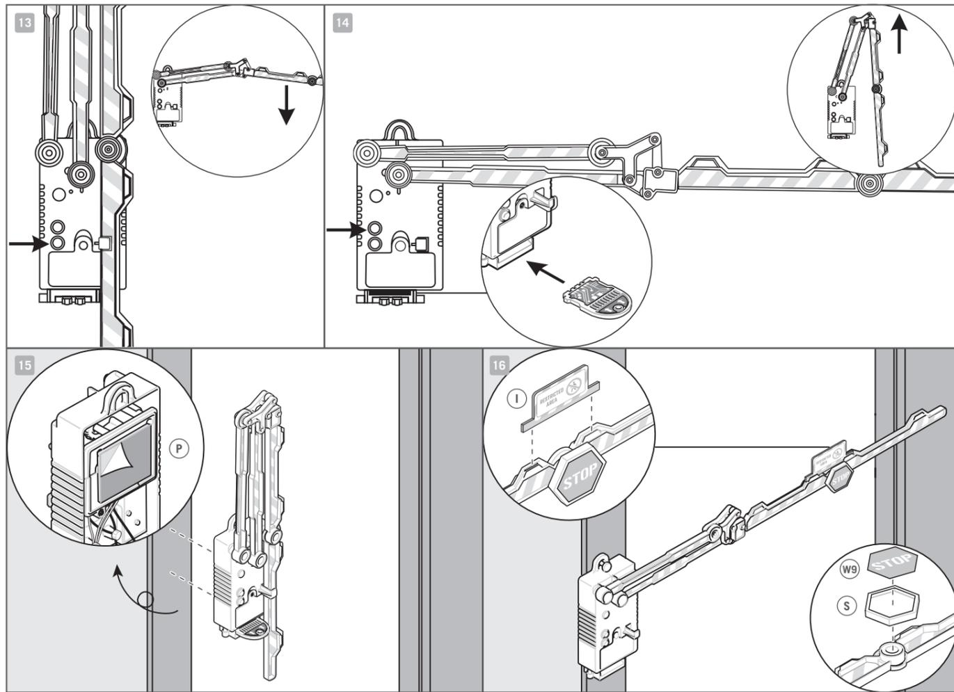
13. Now press the LOWER button and the barrier should extend to block the entrance.
