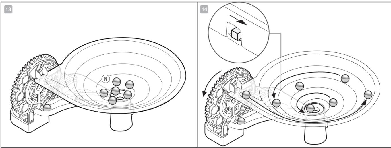
13. Place all the metal balls (part N) in the spiral track. They will roll along the channel in the base until they reach the turning wheel.
