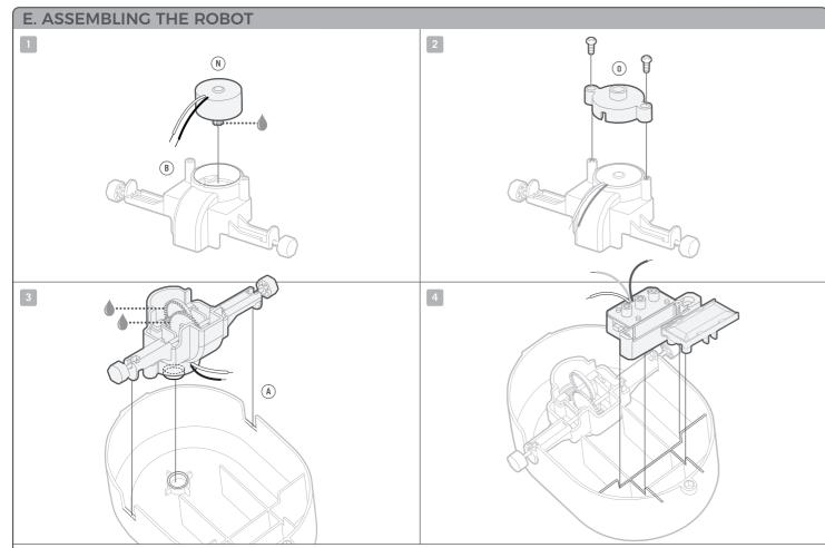
Remark: It is recommended that you apply some lubricant to the joints or moving parts when assembling the product. This helps to reduce friction and enhance mechanical performance. You may use some cooking oil or lotion for this purpose. In the instructions, the "oil drop symbols • indicate the areas which may require lubrication.
