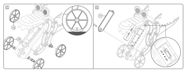
16. Clip two front wheels onto each end of the long plastic axle, and two rear wheels onto the bottom pins on each of the S-shaped links with wing. The triangles marked on the rear wheels should point downwards, so that there is enough friction for the robot to move smoothly.
